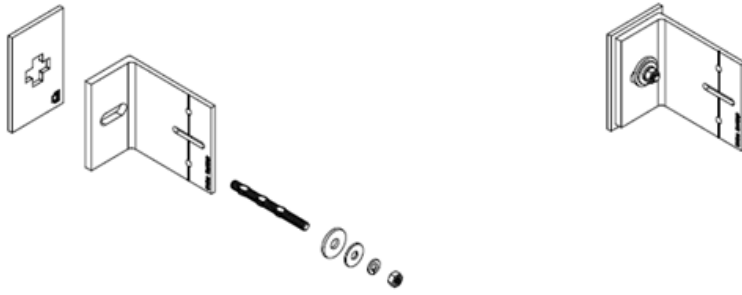
Figure A4.20a: Thermal bridge break piece. Termostop 100.
