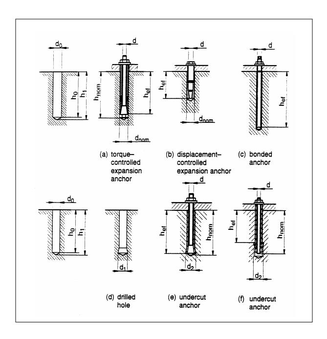
Figure 3.3 Dimensions of drilled hole as well as specific types of anchor
