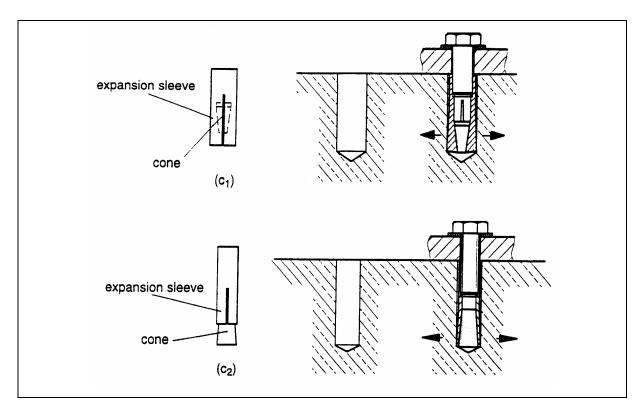
(c) Example of deformation-controlled expansion anchors (Part 4)
