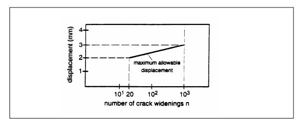
Figure 6.3 Criteria for results of tests with crack movements
