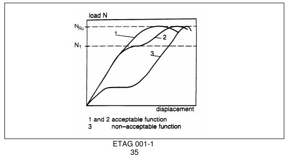
Figure 6.1 Requirements for the load/displacement curve
