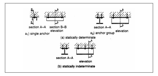
Figure 2.1 Examples of anchored components
