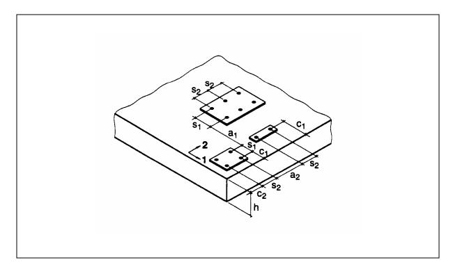
Figure 3.2 Concrete member, anchor spacing and edge distance
