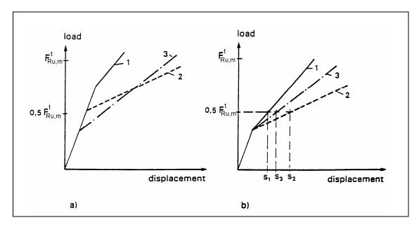
Figure 6.2 Influence of prestressing on load/displacement curves
