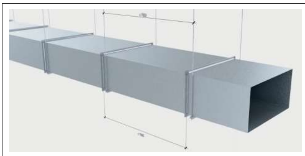
Figure B.1: General view of the steel duct and suspension elements.
