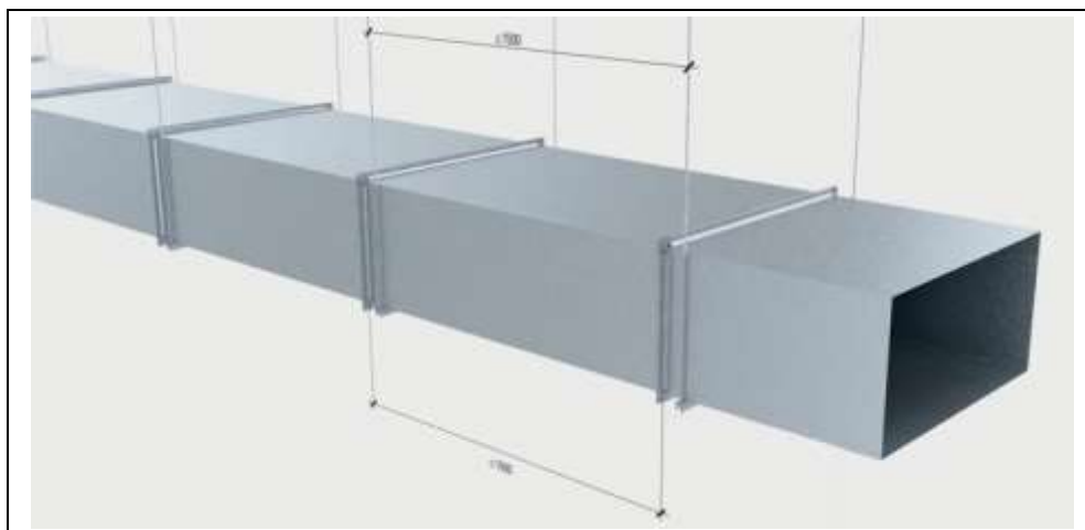
Figure A.1.2: General view of the steel duct and suspension elements.
