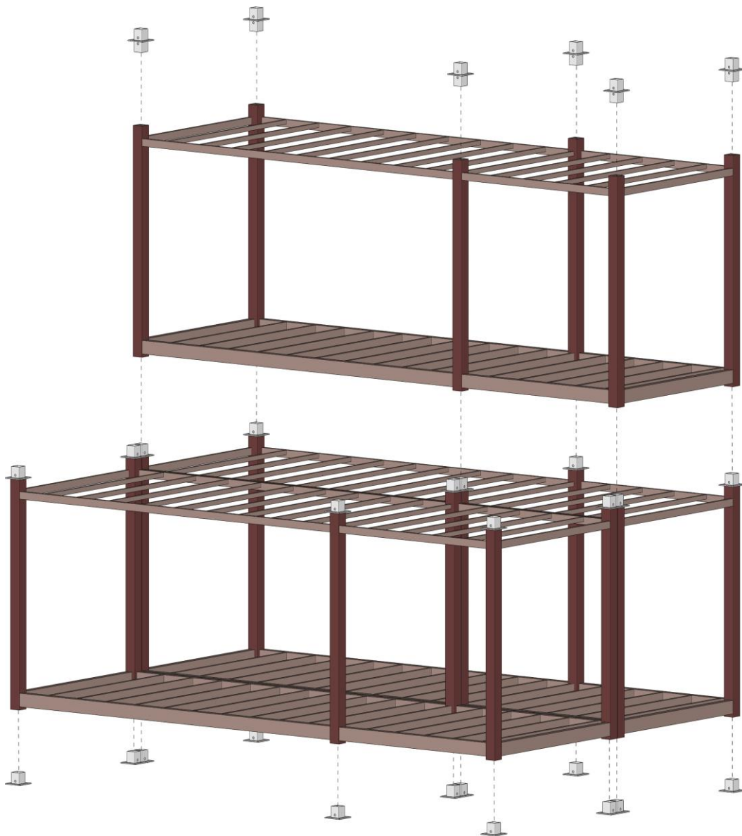
Figure A1.1: SEH ® units, components and connection-pieces.
