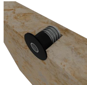
Figure A2.1.3: TR-MASA positioning into the skin element.
