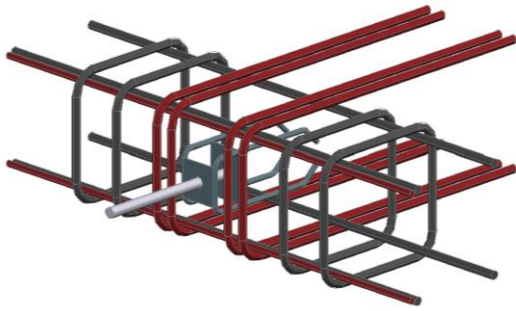
Figure 5.3: Arrangement of the cross-ties of the concrete edge reinforcement and edge beam reinforcement. Three-dimensional view.
